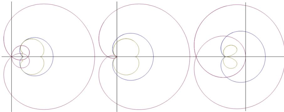
Figure 5: Caustic of the Cardioid : ponctual light at origin
