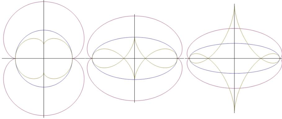
Figure 21: Parallele rays caustics of circle and ellipses
