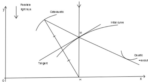
Figure 2: Caustic of a curve for parallele rays to y-axis
