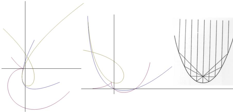
Figure 17: Catacaustics of parabola
