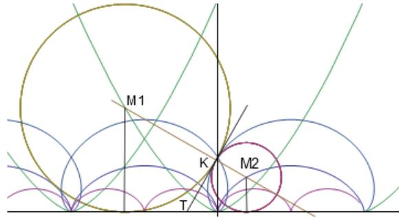
Figure 10: Quadruplet : cycloid/OTT  $\leftrightarrow$  Involute of cycloid and caustic = Cycloid (half size).
