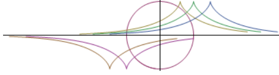
Figure 4: Circles and Tractrix are orthogonal curves for translation along x'x
